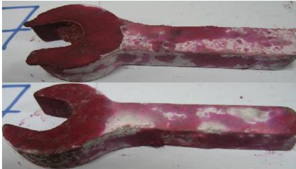
Figure 7: Sample 7 surface defects using PT at PR = 14.9 (cm<sup>3</sup>/s).
