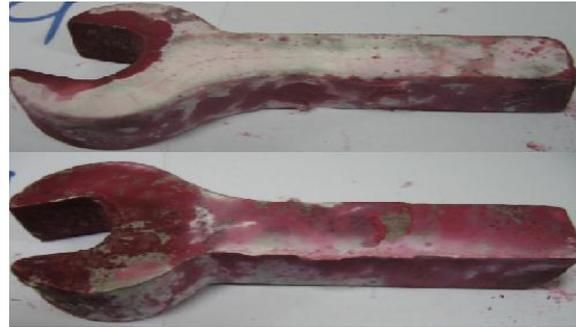
Figure 2: Sample 2 surface defects using PT at PR = 6.3 (cm<sup>3</sup>/s).
