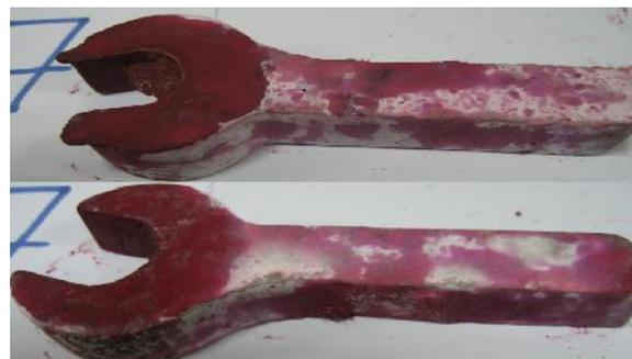
Figure 6: Sample 6 surface defects using PT at PR = 12.7 (cm<sup>3</sup>/s).
