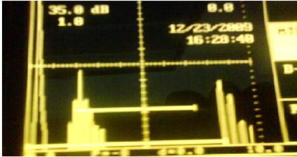
Figure 15: Sample 5 subsurface defects using UT at PR = 12.6 (cm<sup>3</sup>/s).
