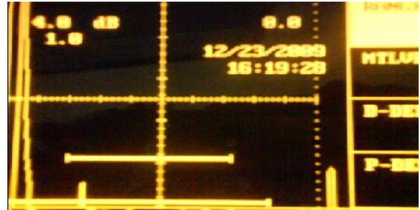
Figure 20: Sample 10 subsurface defects using UT at PR = 24 (cm<sup>3</sup>/s).
