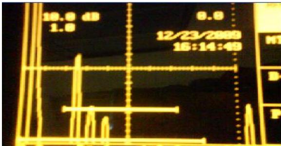
Figure 17: Sample 7 subsurface defects using UT at PR = 14.9 (cm<sup>3</sup>/s).
