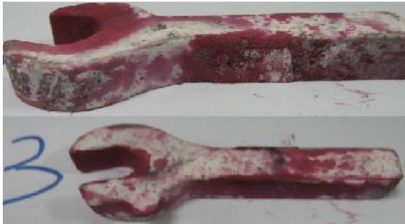
Figure 8: Sample 8 surface defects using PT at PR = 18.6 (cm<sup>3</sup>/s).
