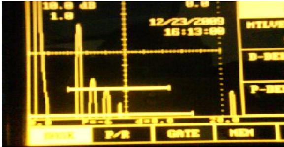
Figure 16: Sample 6 subsurface defects using UT at PR = 12.7 (cm<sup>3</sup>/s).
