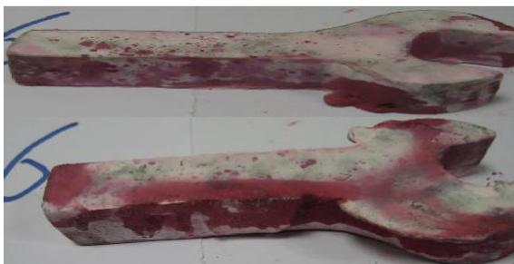
Figure 1: Sample 1 surface defects using PT at PR = 3.4 (cm<sup>3</sup>/s).
