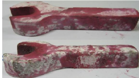
Figure 3: Sample 3 surface defects using PT at PR = 8.7 (cm<sup>3</sup>/s).
