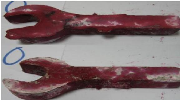
Figure 9: Sample 9 surface defects using PT at PR = 19.2 (cm<sup>3</sup>/s).
